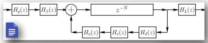
$$H_p(z) = \frac{1-p}{1-pz^{-1}} = \text{pick-direction lowpass filter}$$
